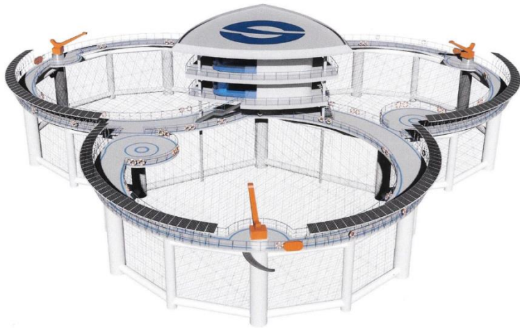
CIMC Blue's Genghai 1, bottom supported offshore cage. Source: CIMC Blue
